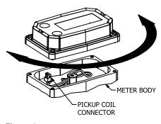
**NOTE:** When rotating the computer display, it is not necessary to disconnect the pickup coil connector, however, care should be taken to avoid inadvertent strain on the connector wires.
